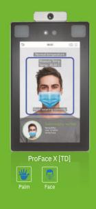
Proface X Series is a fully upgraded version of the Proface product line, which is designed to deal with all kinds of scenarios. Powered by the ZKTeco-customized CPU for running the intellectualized engineering facial recognition algorithm and the latest computer vision technology, the Proface X series supports both facial and palm verification with large capacity and rapid recognition speed, boosting the security performance in all aspects.
